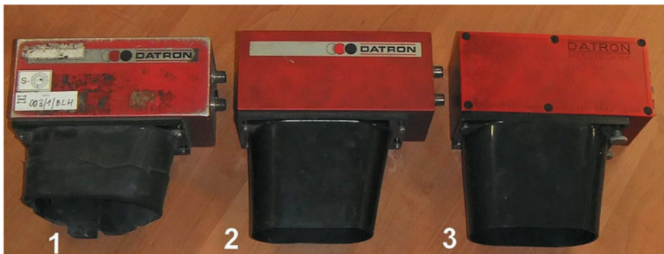
Fig. 1. View of the measuring heads used for tests 1 – Correvit Datron LS1, 2 – Correvit Datron DLS1, 3 – Correvit Datron LM
