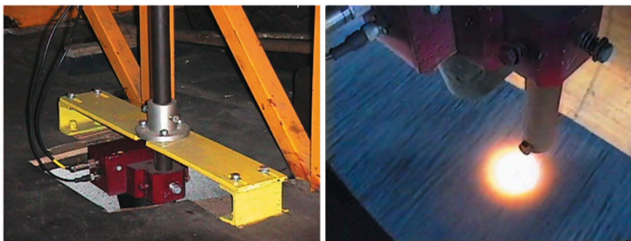
Fig. 7. The measurement head Datron DLS1 mounted in the hole inside the coach's carrier
